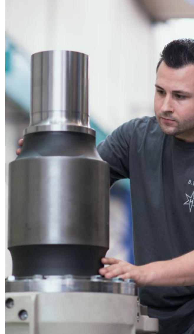
Top drive gearbox for drill drives used in deep drilling technology
