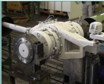
Low temperature test at an AK G 45 gearbox
